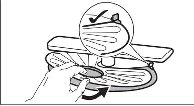
7. Reassemble the filters (B) and (C).
