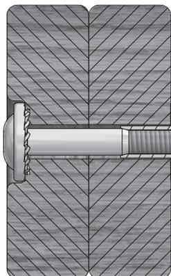
If you see exposed threads and your bolt protrudes beyond the T-Nut you may have over tightened the bolt or used incorrect hardware. If you've overtightened, remove the bolt and add washers to eliminate the protrusion.
