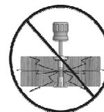
This icon warns you to not over tighten your bolts. This is to prevent structural damage and also splintering your wood.
