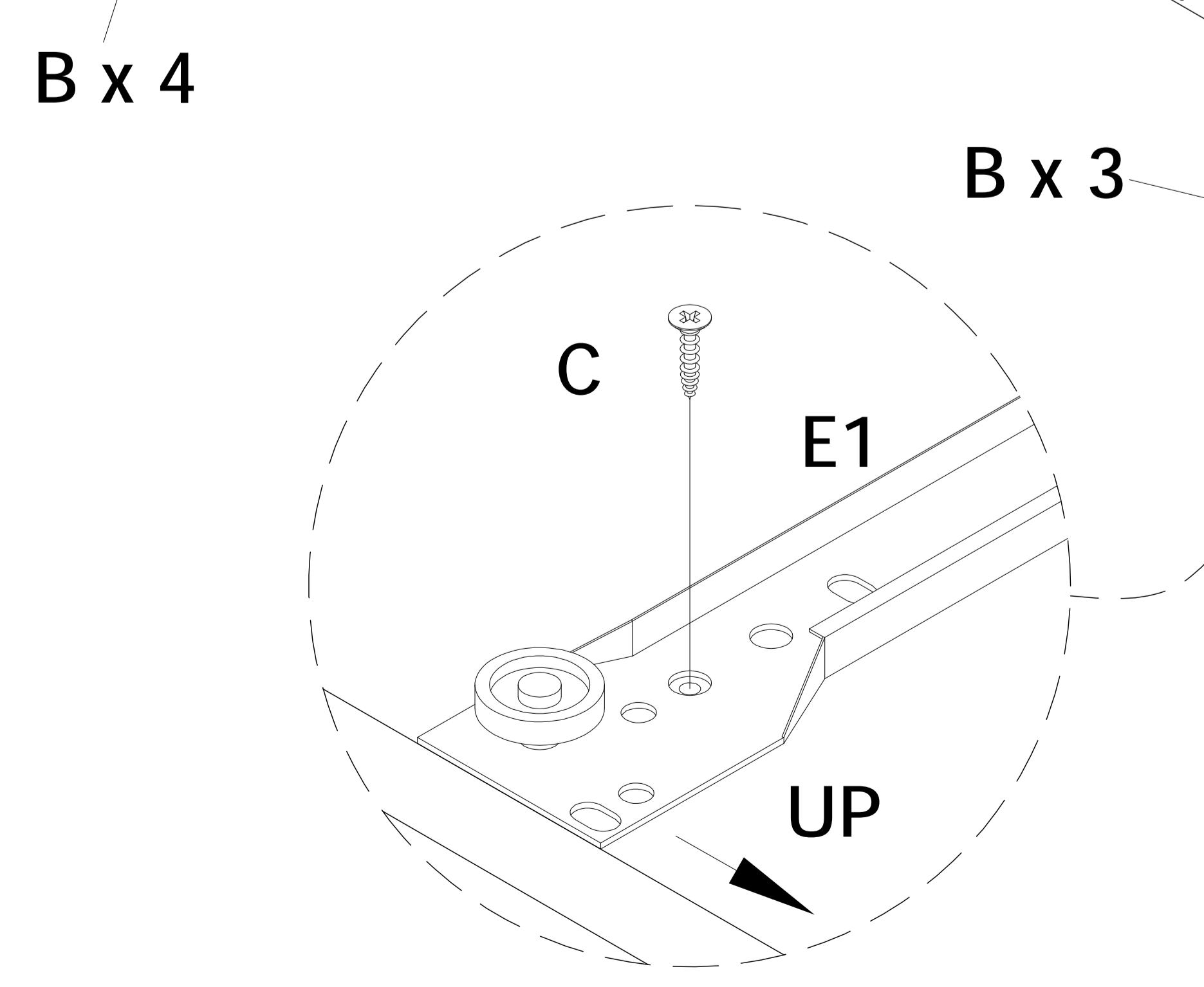
**Hint:** When installing, please make sure the screws are flattened, Not crooked; Otherwise the drawers will not be installed perfectly.
