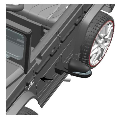
Install reflector: insert reflector in car body hole with a little effort.
