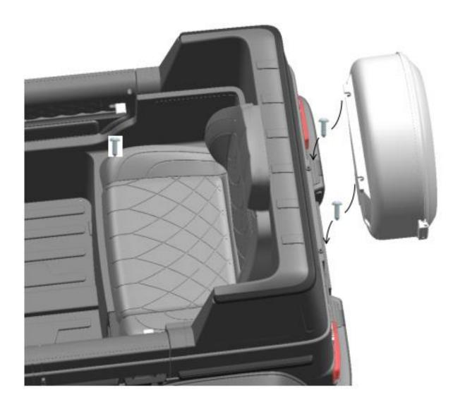
**Install Toolbox:** place the Toolbox on the body and secure it with **2pcsØ 4X12mm** black screws;
