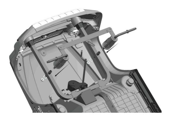
1. As shown, the direction of the front wheel shaft is distinguished, inserted on the support frame, and placed at the bottom of the frame with 1pc gasket, and then fixed with a nut with the front wheel shaft on top of the front wheel shaft;
