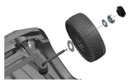
**Install front wheel:** The front axles are fixed with the front axle, and then the front wheels are installed, then the front wheels are placed, and then the front wheels are fixed with a M8 nut. Finally, the wheel core cover is placed on the front axle.
