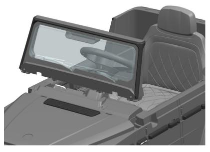
Install the windshield: align the card hole on the vehicle body, and put the windscreen card on the vehicle body by force;
