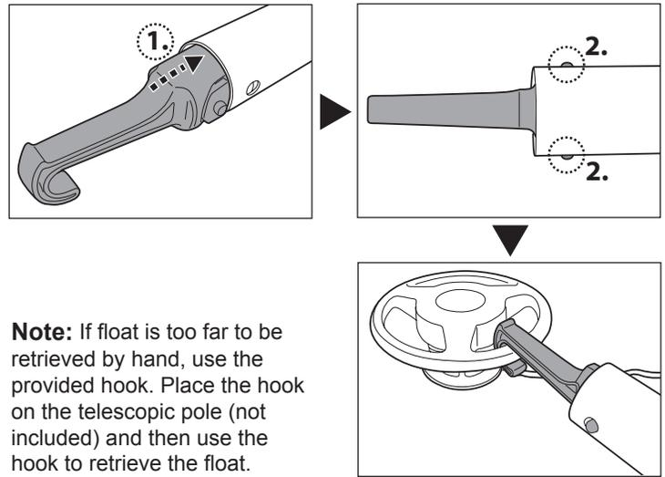
**Note:** If float is too far to be retrieved by hand, use the provided hook. Place the hook on the telescopic pole (not included) and then use the hook to retrieve the float.
