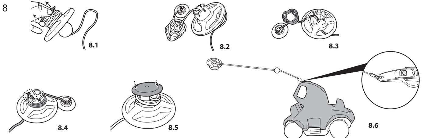
**Note:** Pry to detach the float cover and release the rope from the float to the depth of pool water plus about 0.5m(19.7in.).
