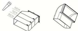
ⓐ—Pipe connector (suitable for cabinets of different widths)
