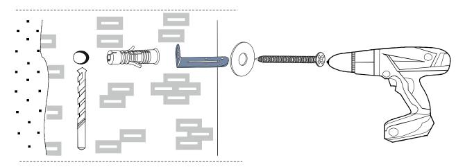
Check the wall type before installation of dowel. Wall is drilled with equal diameter of dowel. (08mm) Universal Plastic Dowel provides the general purpose usage.
