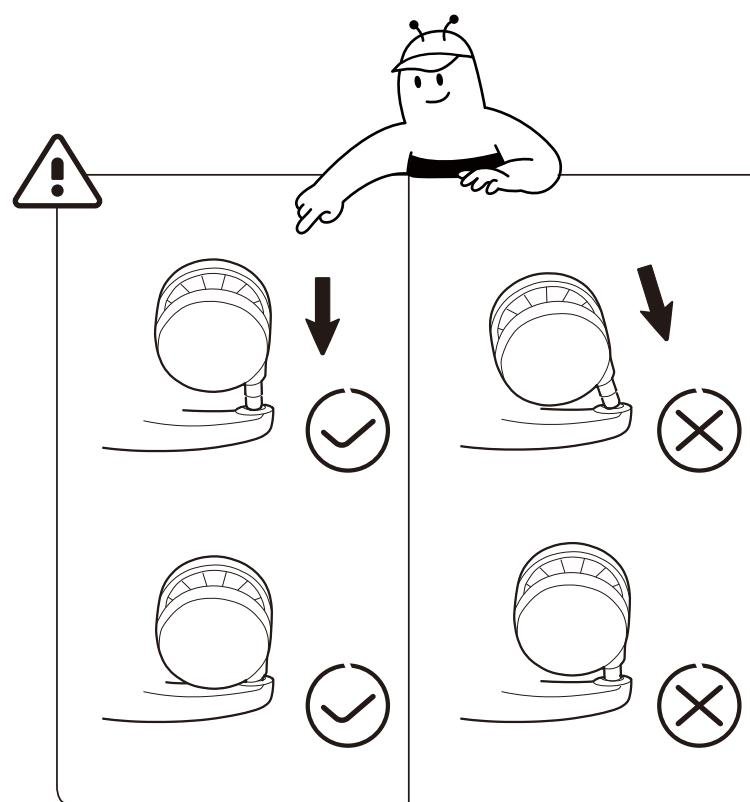
make sure that the axle of the wheel is fully inserted.
