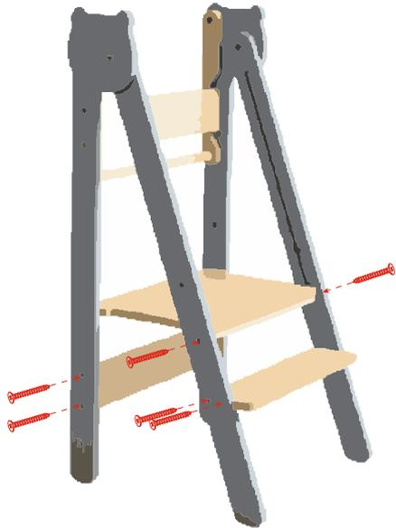
Unscrew the screws on one side only. Only the screws shown in the picture
