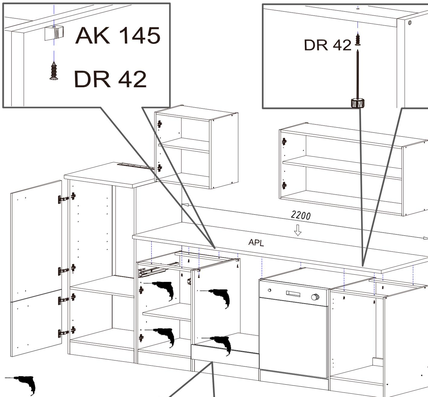
Mit  $\varnothing 5\text{mm}$  Bohrer durchbohren
