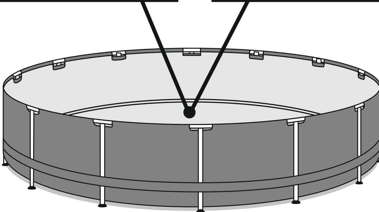
Put 1" to 2" water in the pool to cover the floor. Once pool floor is slightly covered, gently smooth out all wrinkles. Start in the center of the pool and work your way clockwise to the outside.
