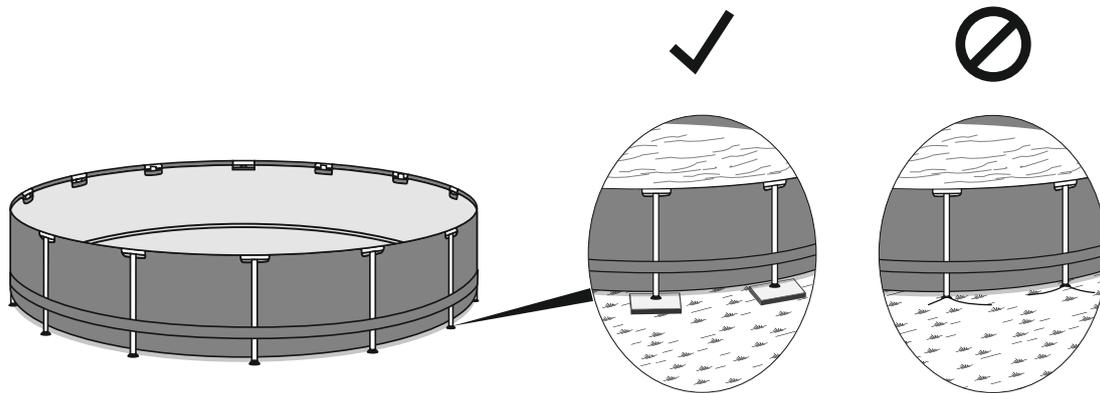
Do not assemble with pool legs on soft lawn. If you must assemble the pool on a soft surface, timber boards (not included) must be placed under the feet of the vertical support rods for even weight distribution.
