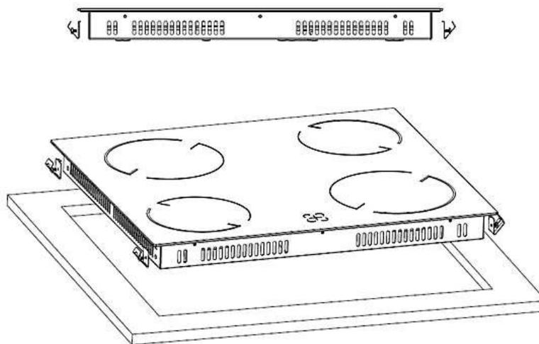
1. Make an installation-opening with the dimensions given on the following drawing (s. **fig. 1**, below).
