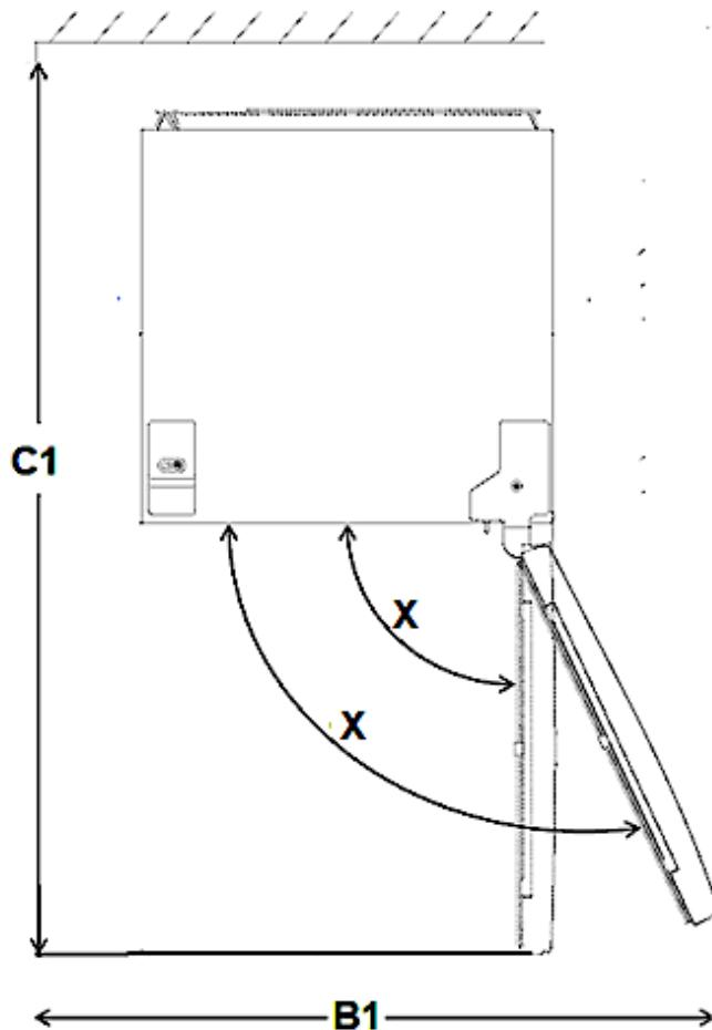
**B1 = WIDTH / C1 = DEPTH / X = DOOR OPENING ANGLE**
