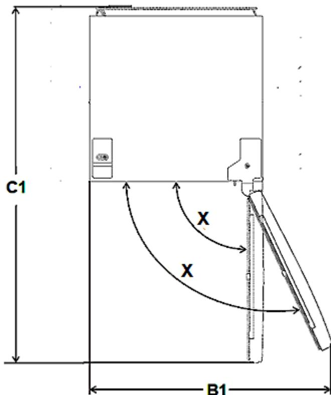
**B 1 = WIDTH / C 1 = DEPTH / X = DOOR OPENING ANGLE**
