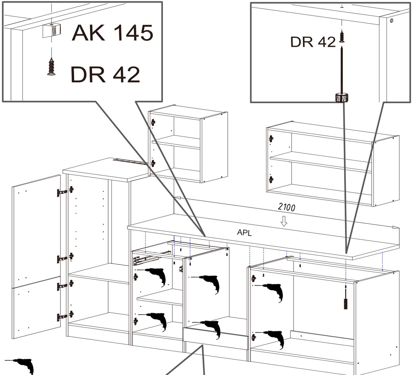
Mit  $\varnothing 5\text{mm}$  Bohrer durchbohren
